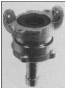
Q.A.C 4 (Forged Steel) Sizes available: 3/8", 1/2", 5/8", 3/4", 1" (Working Pressure=142 psi)
