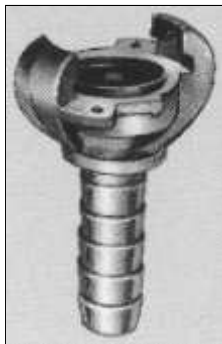
SSI HOSE TAIL (Malleable Iron) Sizes available: 3/8", 1/2", 3/4", 1" (Working Pressure=175 psi)
